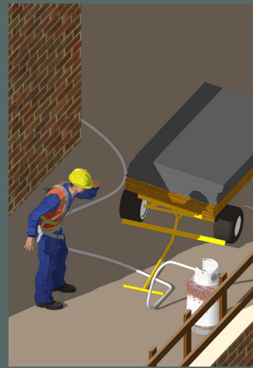
Gas hose (Other conduits, electrical cords, or pipelines can also become obstacles.)
